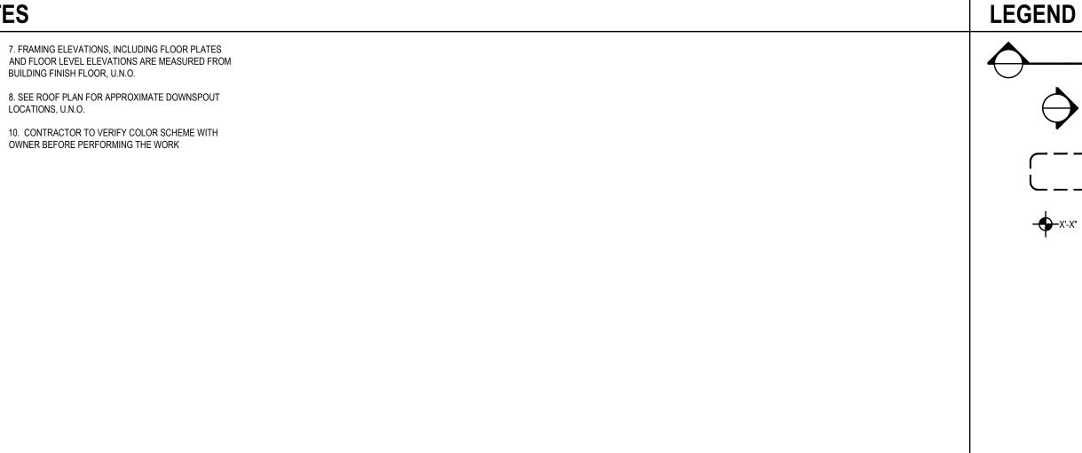
ELEVATION CALLOUT DETAIL DRAWING REF. ELEVATION MARKER
