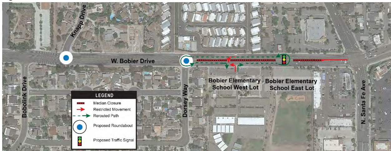
Figure 3-1: Traffic Reroute Illustration
