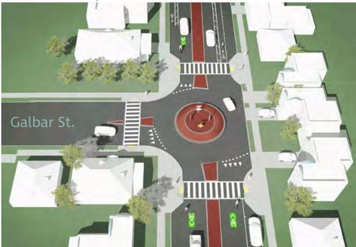
Figure 5-5: Sample 3-way Roundabout
