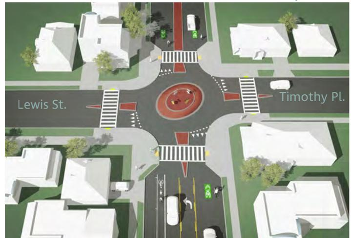
Figure 5-6: Sample 4-way Roundabout
